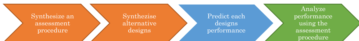
Figure 11 Key steps to completing a trade study. (Orange: Synthesize, Blue: Prediction and Green: Analysis)
