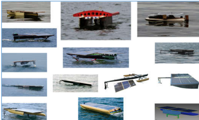
Figure 2 Alternative SolarBoat physical architectures
